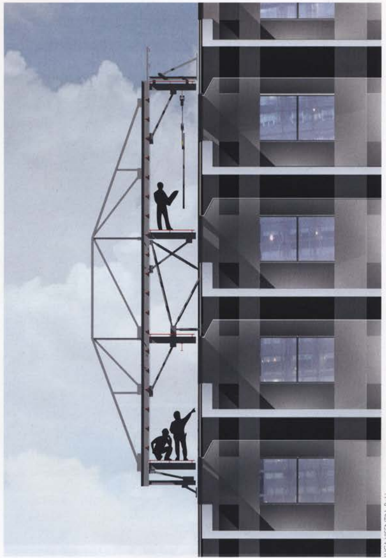
ABOVE A SECTIONAL DRAWING OF THE SUSPENDED ELEVATED PLATFORM ILLUSTRATES HOW THE PLATFORM SYSTEM IS ATTACHED AT THE MIDDLE LEVEL BY TIE-IN STRUTS BOLTED TO TEMPORARY BRACKETS. WINCHES ON THE ROOF SUSPEND THE SYSTEM FROM ABOVE AND MOVE IT DOWN THE FACE OF THE BUILDING USING SLOTS RESERVED FOR THE WINDOW-WASHING EQUIPMENT. WHEN THE PANELS HAVE BEEN INSTALLED, THE TIE-IN STRUTS ARE REMOVED AND THE ENTIRE STRUCTURE MOVES DOWN ONE FLOOR. BELOW, LEFT TO RIGHT TIME-LAPSE CAMERAS RECORD THE PROGRESS OF CONSTRUCTION.
